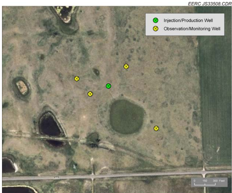
Figure 4. Map of the Burke County study site. Core were collected from the center well which has been designated as a possible CO 2 injection/CBM production well for a future pilot-scale ECBM project.
