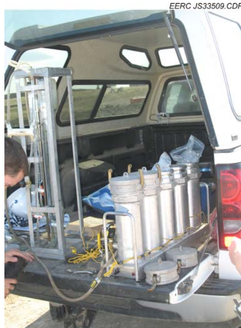
Figure 6. Canisters and apparatus used in the field to maintain core samples at reservoir conditions as part of the gas content analysis procedure.
