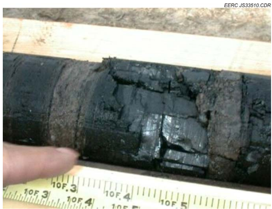
Figure 5. Photograph of Burke County lignite coal core immediately after collection and prior to placement in canister for gas content analysis.
