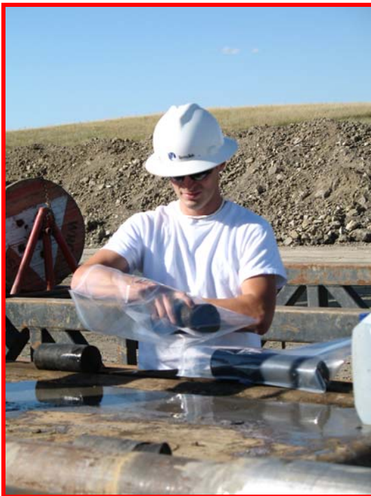
Figure 4 – Photograph of the core being prepared for canister testing.
