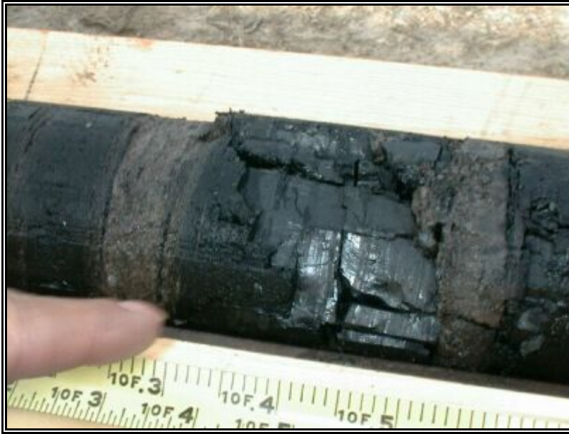
Figure 3 – Close-up photograph of the lignite coal core collected in Burke County, North Dakota.
