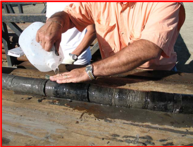
Figure 2 – Photograph of the coal core sample immediately after collection. The sample is being rinsed prior to the initiation of canister testing for gas content analysis.
