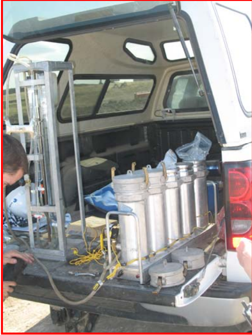
Figure 5 – Photograph of the canister testing apparatus used to initiate gas analysis activities in the field immediately after collection of the lignite core sample.
