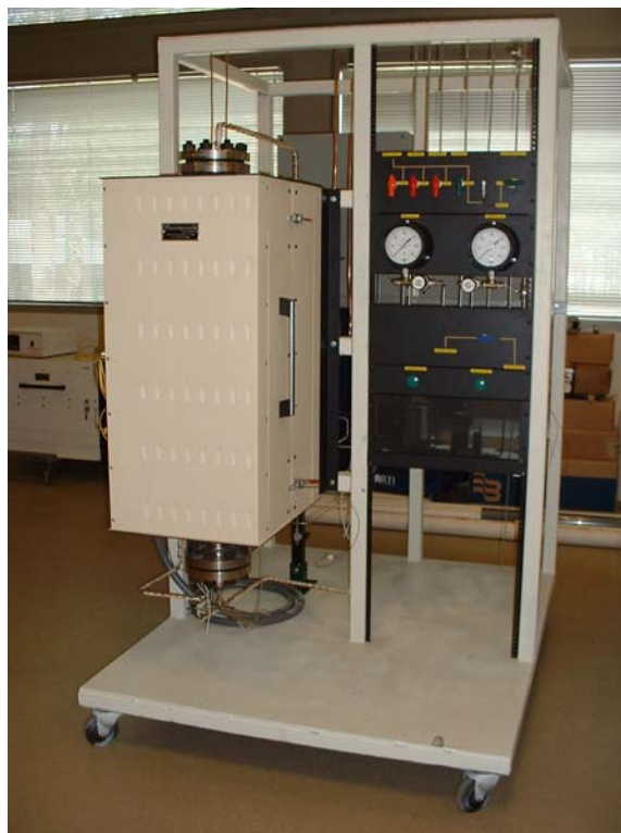
Figure 27: Photograph of the pilot-scale test skid. The picture also shows a three-membrane tube module housed inside a 36"-long three-zone furnace.
