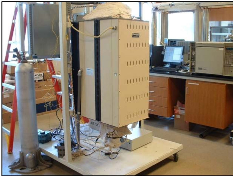
Figure 31. Functional pilot-scale skid with GC and computer control system.
