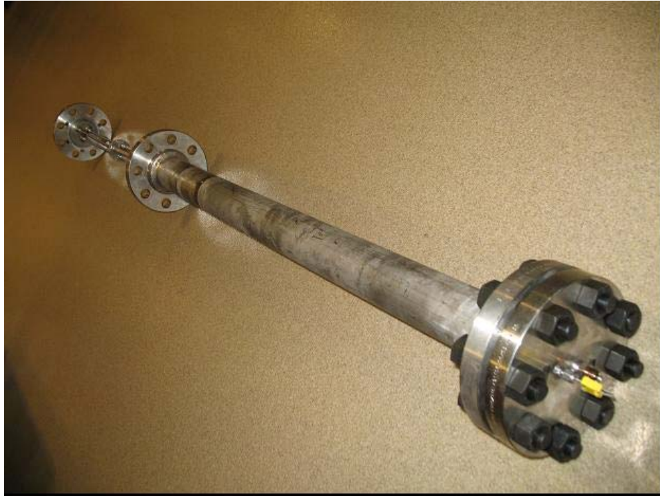
Figure 29. Housing shell for multi-tubular module, 2.5" ID, 42" length.
