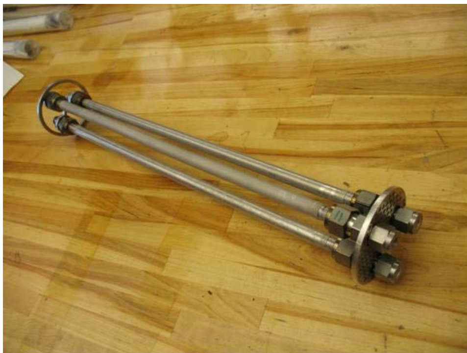
Figure 28. Three-tube membrane module held between two rings and Swagelok fittings.
