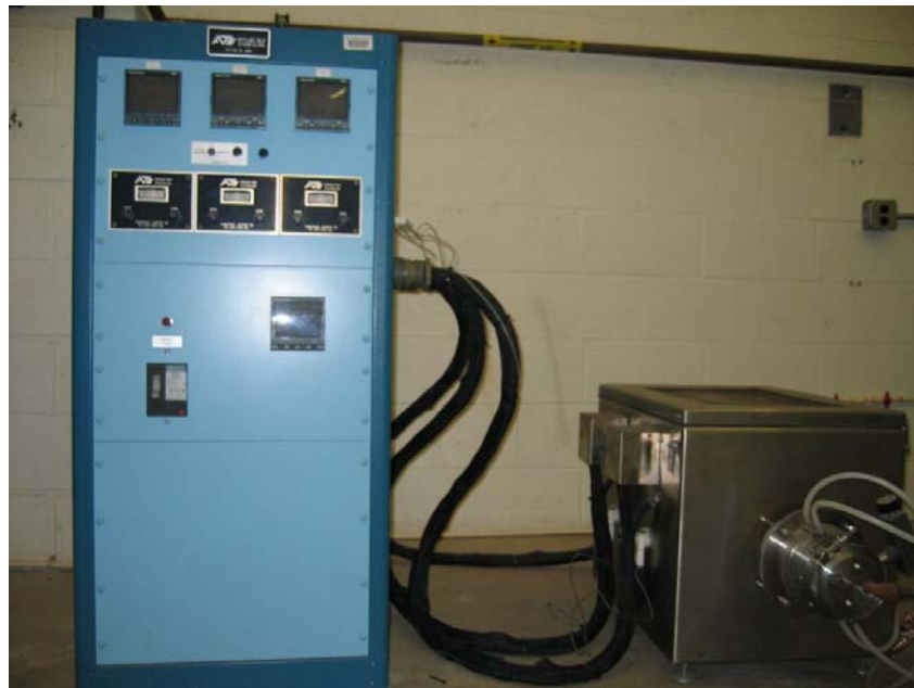
Figure 2: The Directional Solidification (DS) furnace at WVU.
