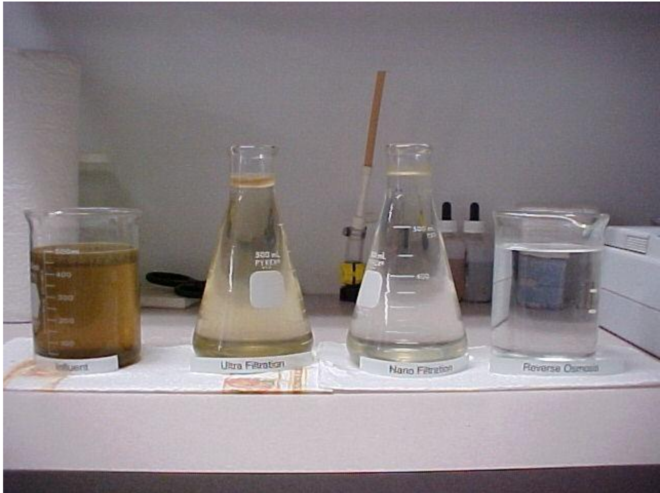
Figure 3: ESTR Pilot Trial Membrane Filtration Water Sample Results
